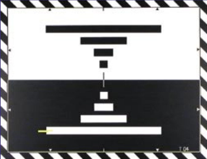
Bar Test Chart showing area of overshoot measurement.
