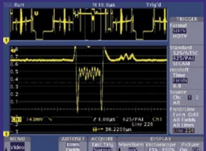
Bosch Dinion XF LTC0610 colour camera resolution waveform showing about 15% depth of modulation at 480 TV lines.
