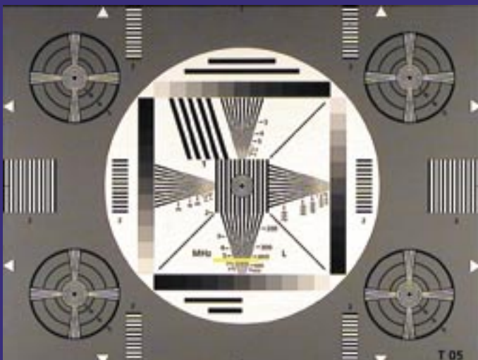
Universal camera test chart (RETMA) image showing area of resolution measurement.
